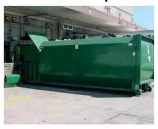
Compactors are machines that are used to compress large quantities of general mixed (unsorted) or sorted recyclable waste into tightly packed blocks, which are then sent to a recycling company or landfill. With an industrial commercial compactor, your company's recycling process becomes easier and more profitable.
